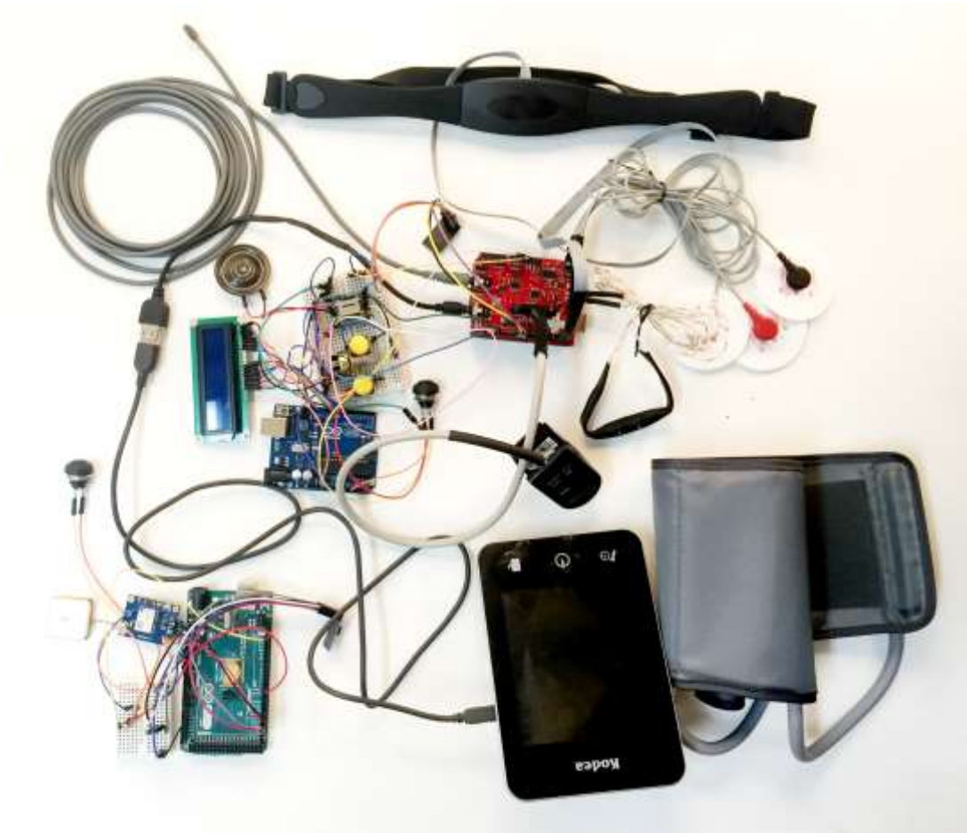
Figure 2: Hardware Setup of the Remote Patient Monitoring Prototype
